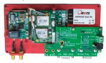
Evaluation Kit - plate mounted xOEM and breakout board
